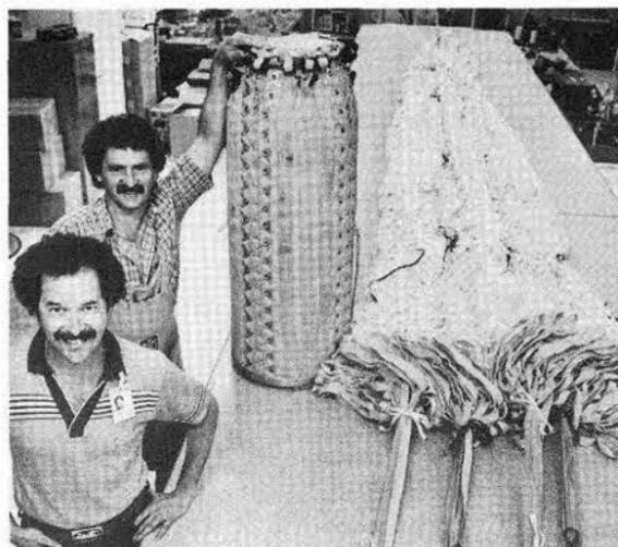
AT SANDIA'S PARACHUTE LAB, Kenneth Ronquillo (front) and Richard Brazfield (both 1632) prepare a 70-foot-long B83 parachute for packing. Completed pack is 16.5 inches in diameter and 42 inches long. It weighs 225 pounds.
